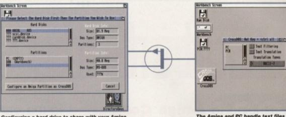
Configuring a hard drive to share with your Amiga and PC is as easy as pointing and clicking your mouse thanks to this utility The Amiga and PC handle text files in radically different ways. This utility automatically converts between the two types when copying
